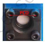
Measure the center distance of any bolt hole where the valve block is installed, and then check it.
